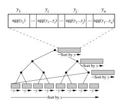
Figure 8: Divisible Aggregates in a Layered Range Tree
