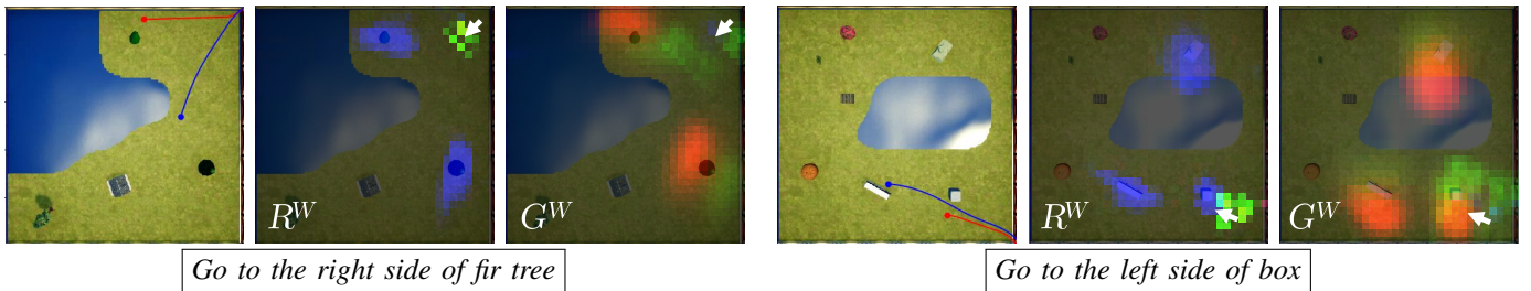
Fig. 6: Two task failures using our approach. The ground truth and policy trajectories are shown in red and blue respectively. On the left, the failure is due to an ambiguous instruction. The Relevance Map R^W overlaid on the environment reveals that the agent has correctly grounded the instruction to the two fir trees present, while ignoring the other objects. The goal map G^W shows that the goal location is inferred for both fir trees. The agent correctly reasons about the task, but the ambiguity confuses it. On the right, box is incorrectly grounded to multiple objects as seen in R^W . Given this wrong grounding, the goal location is inferred to the correct side (left) of all grounded objects, as shown in G^W . The agent then executes given the confused goal map, which causes it to fly through the correct goal and towards one of the wrongly detected goals.
