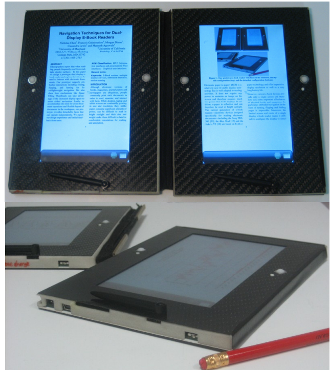
Figure 1 - Our prototype e-book reader with faces in the attached, side-by-side configuration (top), and the detached configuration (bottom).
