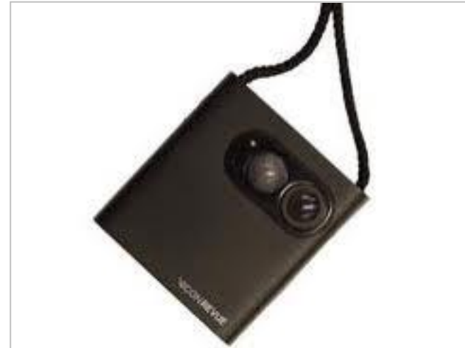
figure 1. The SenseCam lifelogging device, now commercially named the Vicon Revue.
