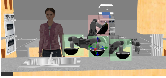
Figure 1: Our user feedback system. Different trajectories are shown to users to select from. In this example, interactive feedback allows a user to move waypoint 2 (in red) to waypoint 3 (in green). Waypoint 3 shows interactive markers that guide the user.
