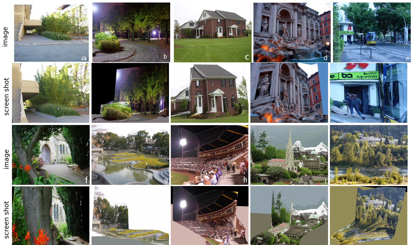
Figure 9. Typical results from our algorithm. Original image (top), and a screenshot of the 3-d flythrough generated from the image (bottom of the image). The first 7 images (a-g) were evaluated as “correct” and the last 3 (h-j) were evaluated as “incorrect.”
